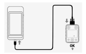
Figure 11-1 Connecting MaxiTPMS Tablet and Hand-held Inclinometer
