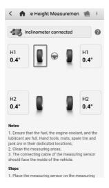
Figure 11-3 Ride Height Measurement Result Screen
