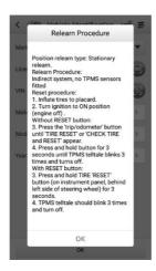
Figure 5-8 Relearn Procedure for Indirect TPMS
