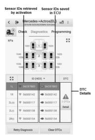
Figure 4-12 CV Diagnostics Screen
