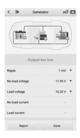
Figure 8-12 Generator Test Result Screen
