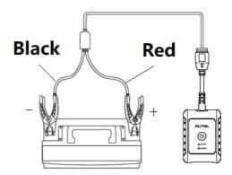
Figure 8-2 Connecting to a Battery
