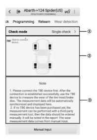
Figure 5-33 Wear Detection Screen
