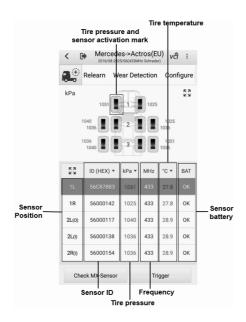
Figure 4-10 CV Check Screen
